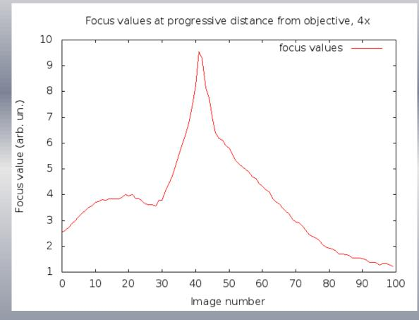
For example, this is a graph of the focusing values of a sequence of images taken at equal distances, going downwards from the objective. The position corresponding to the peak is the focus point.
